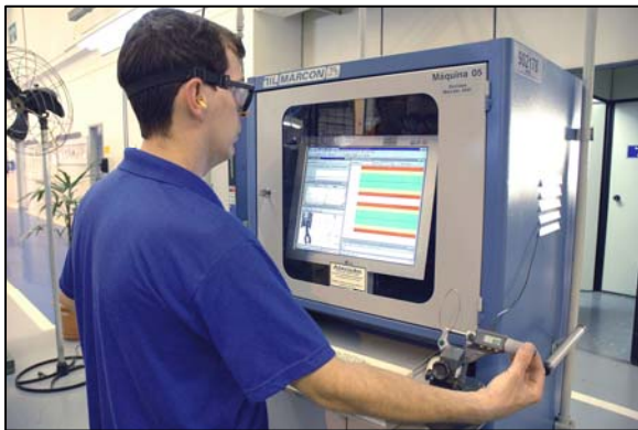
Figure 4. An operator inspects a piston ring using Applied Stats.
