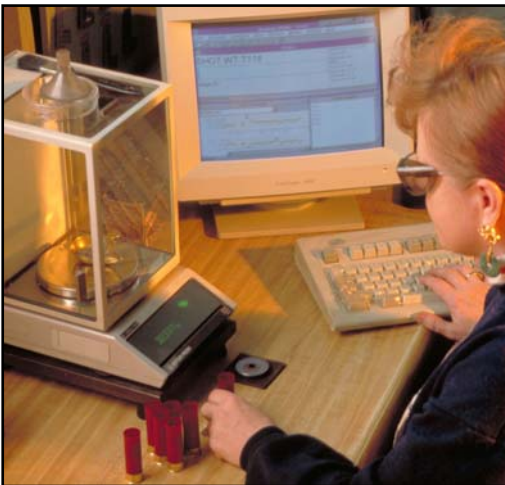
Samples from the Shotshell line are weighed and data is recorded using Quantum SPC/DC.
