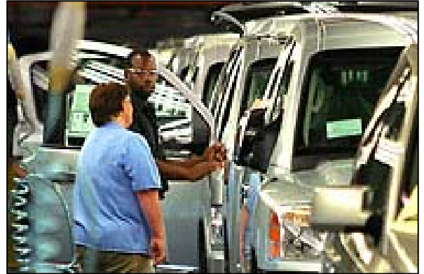
Inspectors discuss problems with binding outside mirrors on sport utility vehicles coming down the assembly line.
