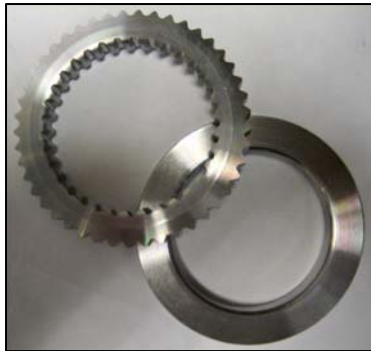
Gearsets are turned from bar stock on the three lathes on the new line.
