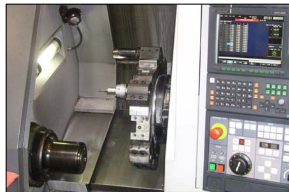
Probes are mounted directly on the turret to measure the X and V axes of the bar stock being fed into the lathe.
