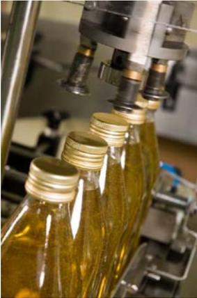
Implementing an SPC and Net Weight control system using DataMetrics software is the first step in recovering some of this overfill. By collecting data from weigh scales and other instrumentation at the point of production, the company can see changes in the process as they occur and take action immediately to resolve the problem.
